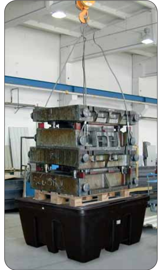
PE-KT-1S under a test load of 8.000 kg
