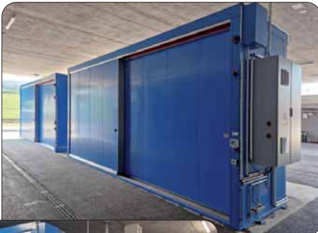
◆ Small aisle width due to the use of sliding gates
