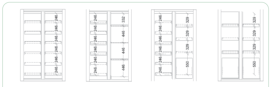
SiS Type 90 / 1200 ES MI, Article no. B80-2556-B, RAL 7035, incl. 6 pull-out shelves (left), 3 pull-out shelves and 1 disposal compartment (right)
