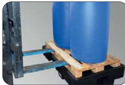
Safe positioning of the Euro pallet
