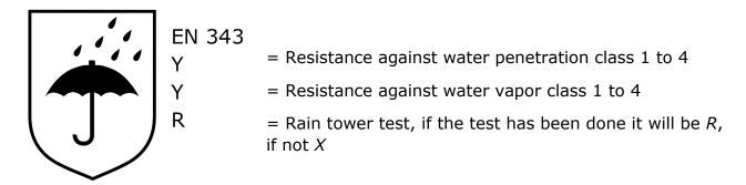
The clothing has achieved EN 343:2019 class 4 for resistance against water penetration and 1 for resistance against water vapor.
